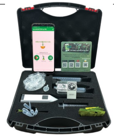
The biometer is a comparison test. Producing a number representing the bio-mass of fungi and bacteria.
